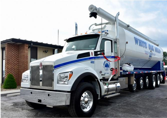
According to Long, the truck can deliver full loads of feed via a top mounted auger system that sends feed to storage bins. In addition, the truck is equipped with a vacuum for grain recovery. “Oftentimes, we will have a customer who wants to move excess feed to another bin or farm,” explained Long. “With this unit, we can vacuum up the feed, then transport and offload. It’s our do-all truck and will keep busy.”
