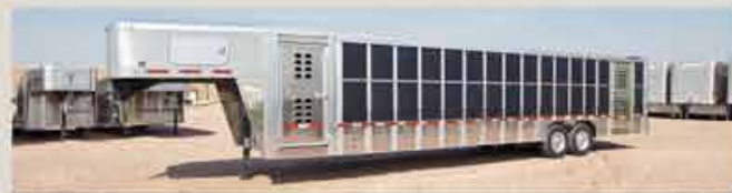
Extruded Aluminum Post Side Construction with Cold Weather Panels
