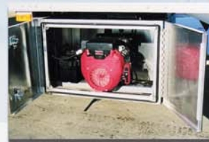
20 H.P. Gas Unload System
