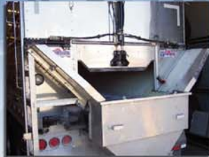
Aluminum Grain Funnel with optional Product Deflectors
